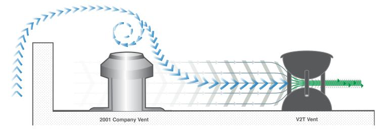
The second difference is the positioning and principles of operation of the two systems. Because Kelly system is designed to operate in the negative zone, the vents are best positioned on the perimeter edge. However, that makes the vents on the non-windward side far less effective, and potentially non-operational.
