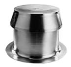
The V2T Vent Technology geometry has a vent design that utilizes the Venturi principle through the opposing two hemispheres that will accelerate the wind through the vent. This now creates a negative pressure that is greater than the uplift pressure that is being exerted on the roof. In most cases, these vents will be positioned approximately 20-25' from the perimeter where the wind coming over the perimeter will reconnect to the roof surface and be accelerated through the vent.
