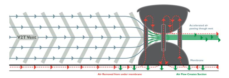
The turbine vents of the 1980s were on to something with the concept of moving air – but it wasn't quite hitting the mark. What if it was a low-wind day? V2T's answer was to employ the Venturi principle to create a vacuum effect.
