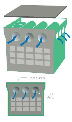
It was a simple, yet effective solution. Air passed above and below the main roofing surface at close to equal speeds as there were no obstacles slowing the wind above or below enough to make a meaningful differential in pressure or lift.
